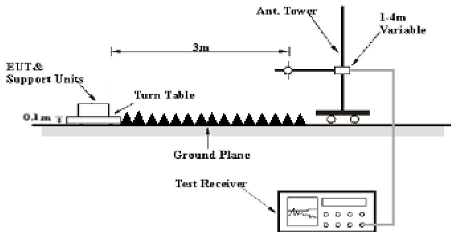
The radiated emission tests were performed in the 3 meters chamber test site, using the setup accordance with the ANSI C63.10-2013. The specification used was the FCC 15.209, and FCC 15.247 limits. The external I/O cables were draped along the test table and formed a bundle 30 to 40 cm long in the middle.
