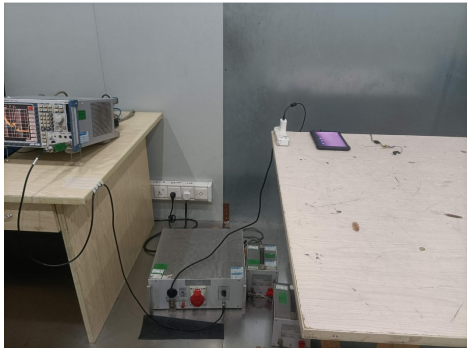
Conducted Emission Test Setup
