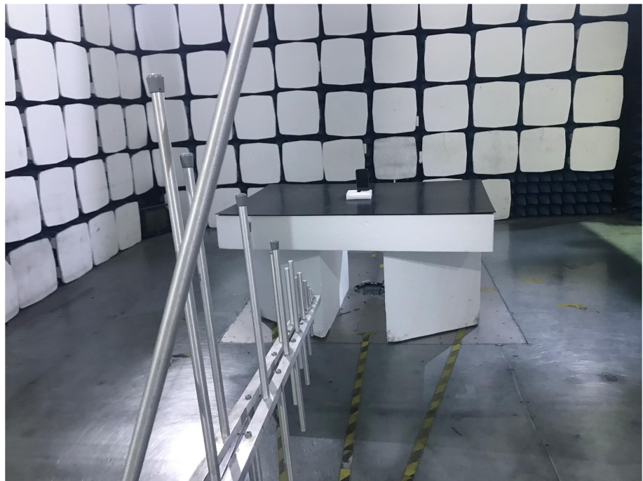
Radiation Emission Test Setup (30MHz to 1GHz)
