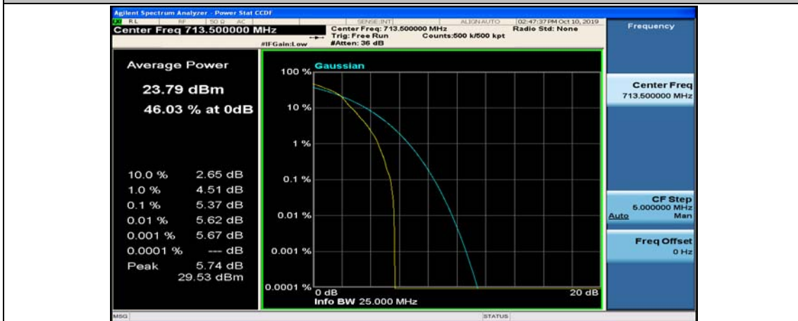
(Channel Bandwidth: 5 MHz)_HCH_16QAM_1RB#12
