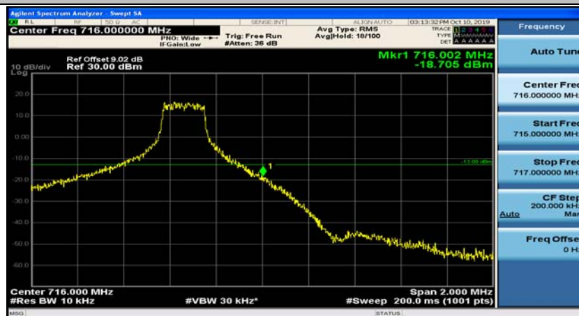
(Channel Bandwidth: 5 MHz)_HCH_16QAM_12RB#0
