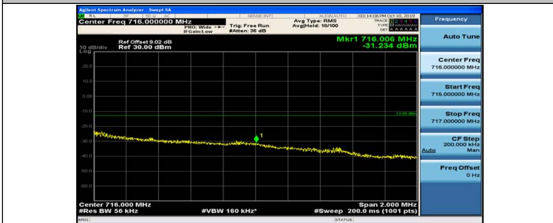
(Channel Bandwidth: 5 MHz)_HCH_16QAM_12RB#13
