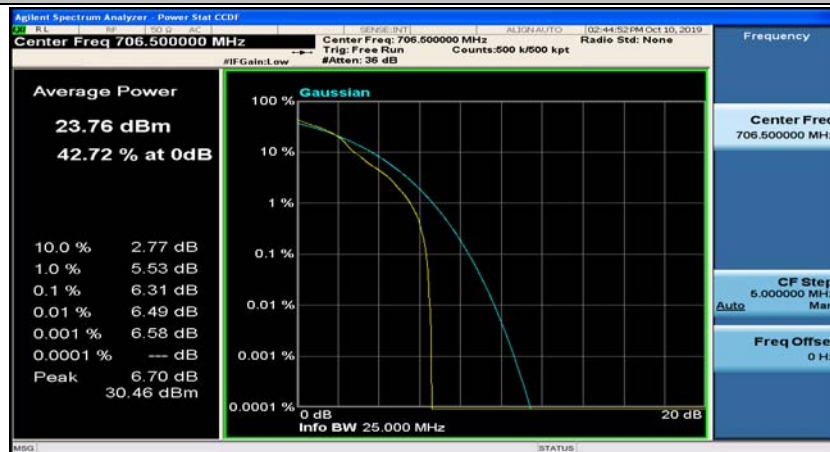
(Channel Bandwidth: 5 MHz)_LCH_16QAM_12RB#0
