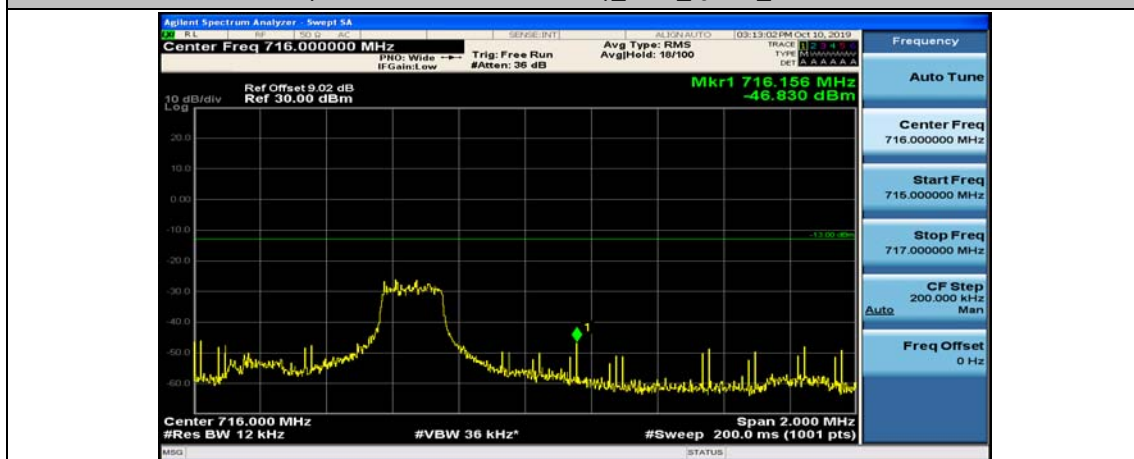
(Channel Bandwidth: 5 MHz)_HCH_QPSK_1RB#12
