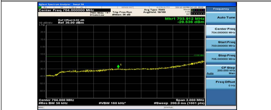
(Channel Bandwidth: 5 MHz)_LCH_QPSK_12RB#13
