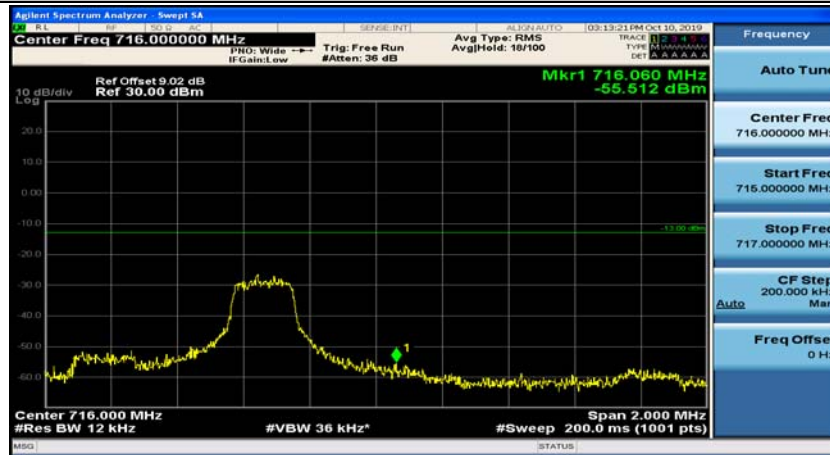
(Channel Bandwidth: 5 MHz)_HCH_16QAM_1RB#12
