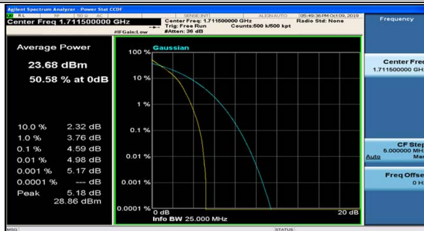
(Channel Bandwidth: 3 MHz)_LCH_QPSK_8RB#7
