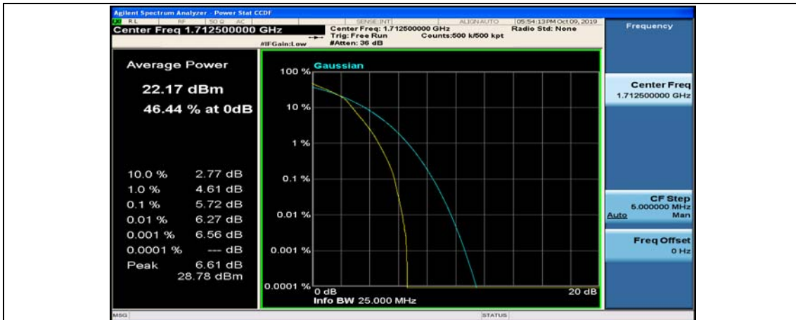
(Channel Bandwidth: 5 MHz)_LCH_16QAM_25RB#0
