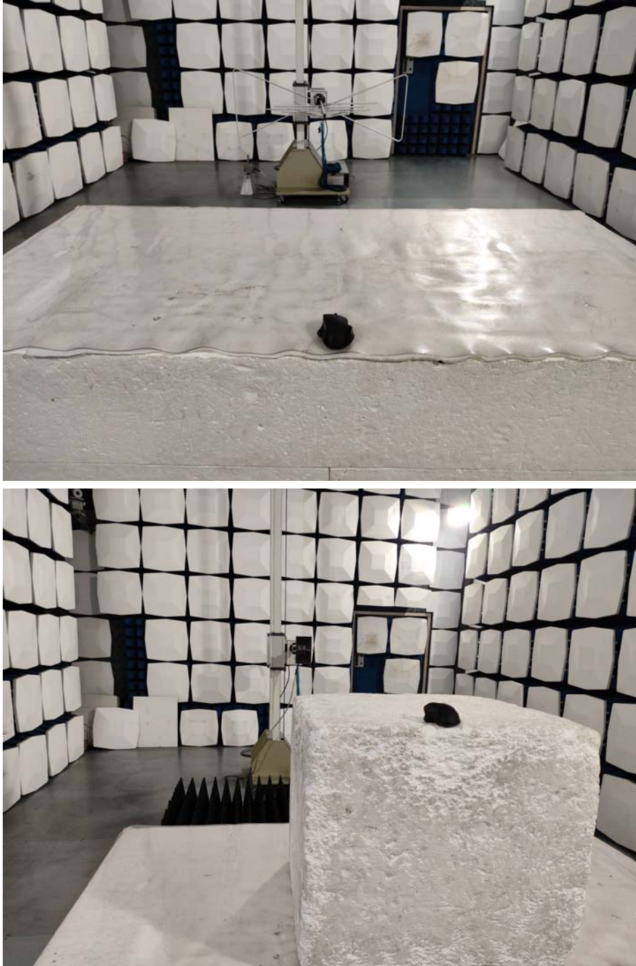
Radiated emission test view
