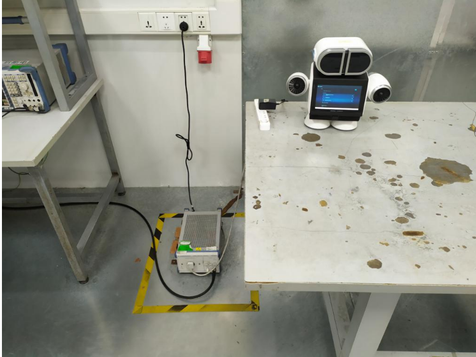
FCC ID:2AH9Q-MDCK00101R Photo of Conducted Emission Measurement
