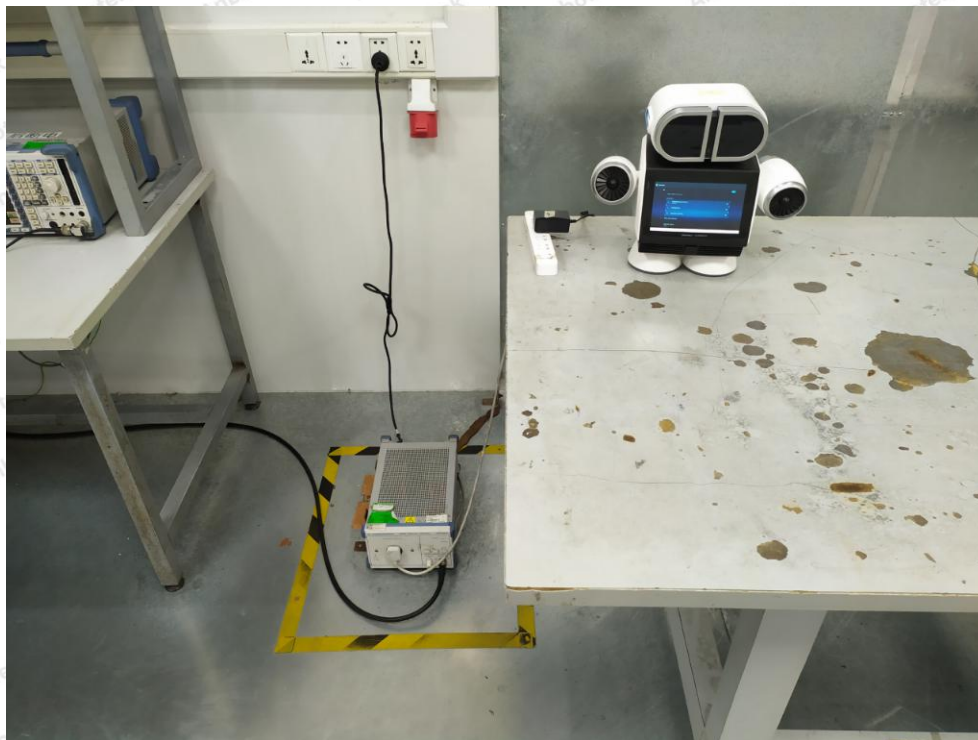
Photo of Conducted Emission Measurement
