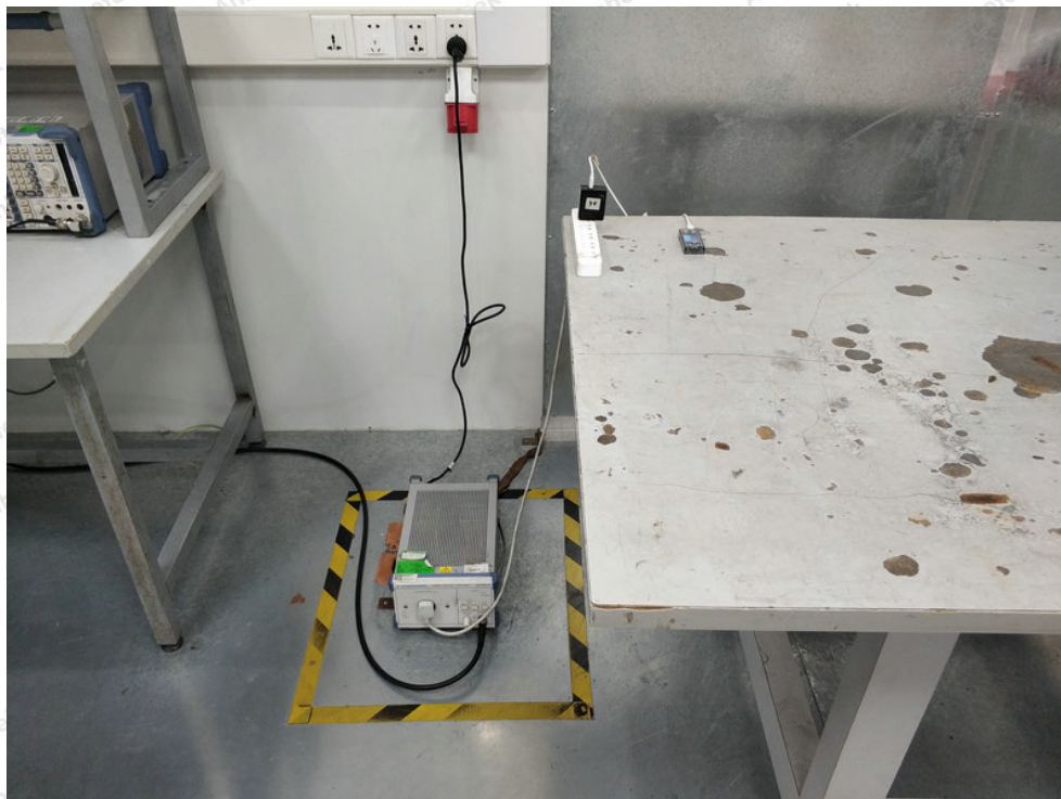
Photo of Conducted Emission Measurement
