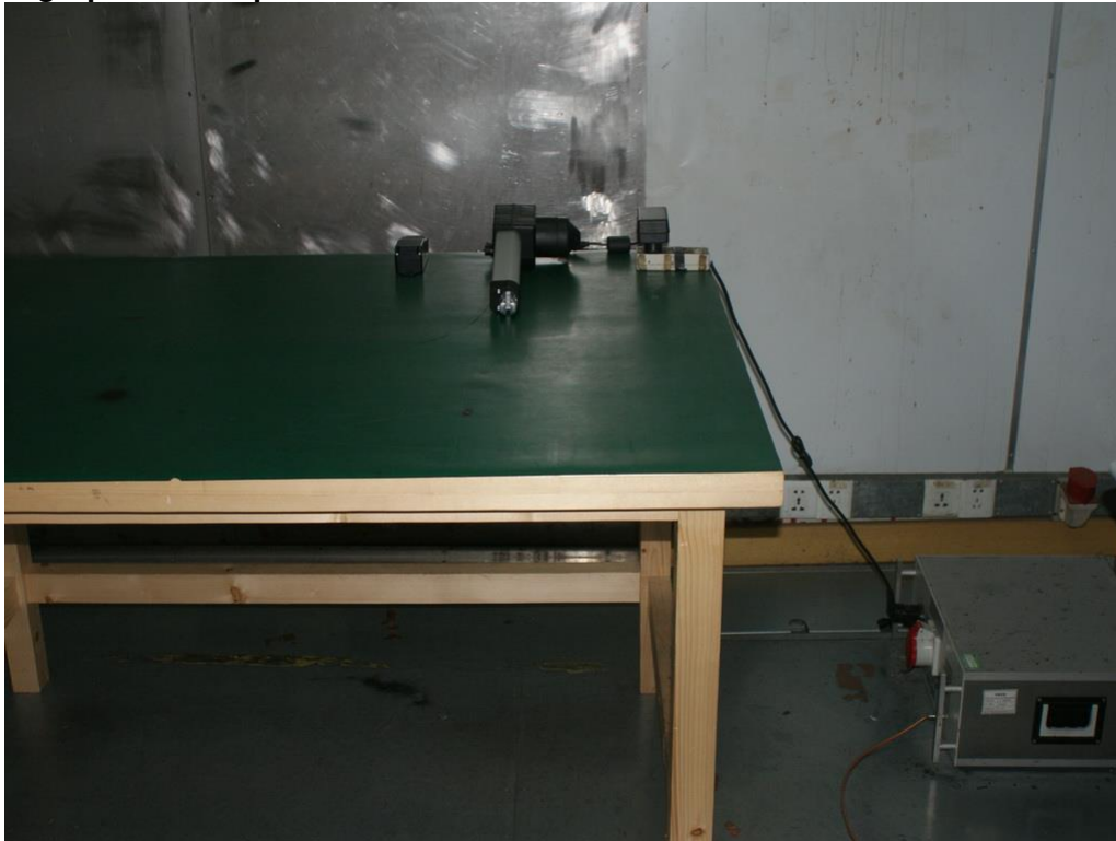
Photograph 5: Set-up for Conducted Emission
