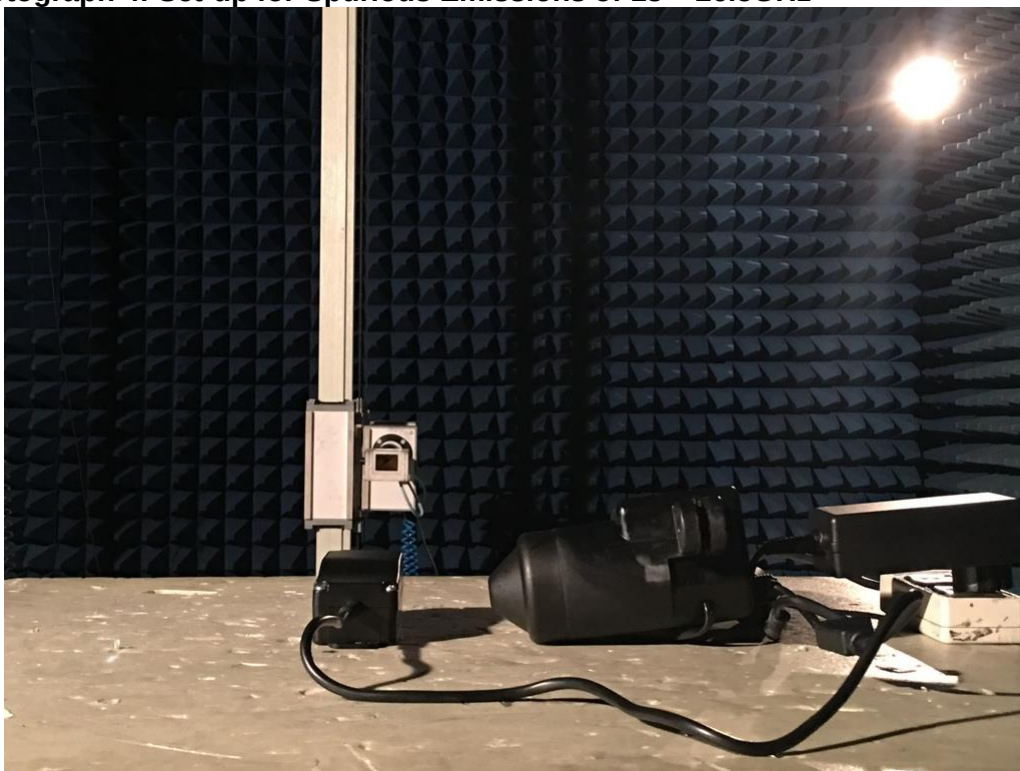
Photograph 4: Set-up for Spurious Emissions of 18 – 26.5GHz
