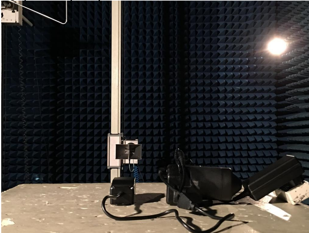
Photograph 4: Set-up for Spurious Emissions of 18 – 26.5GHz
