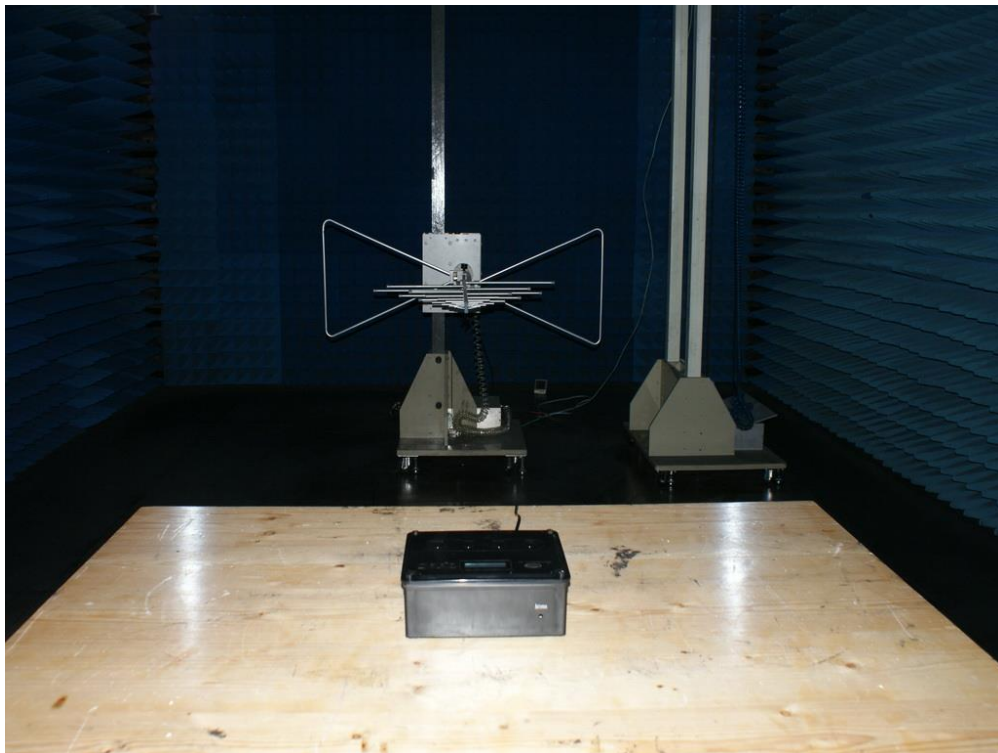
Photograph 2: Set-up for Spurious Emissions (30MHz-1GHz)
