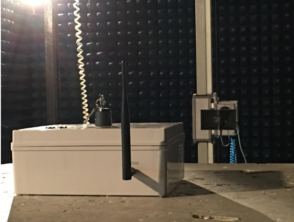
Photograph 4: Set-up for Spurious Emissions of 18 – 26.5GHz
