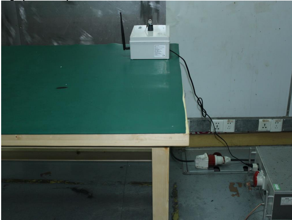
Photograph 5: Set-up for Conducted Emission
