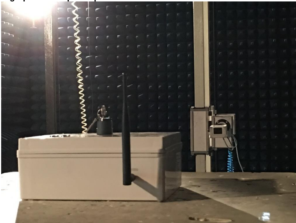
Photograph 4: Set-up for Spurious Emissions of 18 – 26.5GHz
