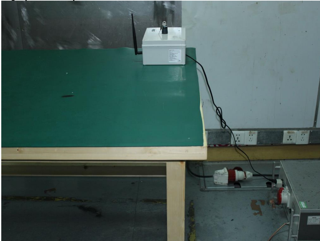
Photograph 5: Set-up for Conducted Emission
