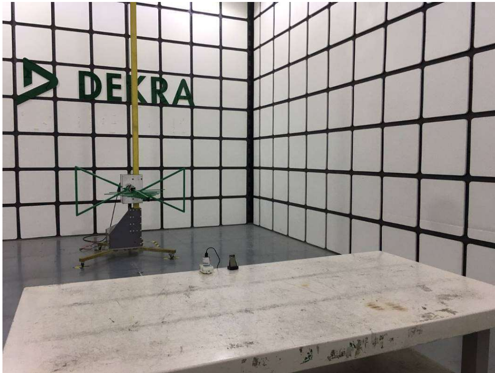
Radiated emission test
