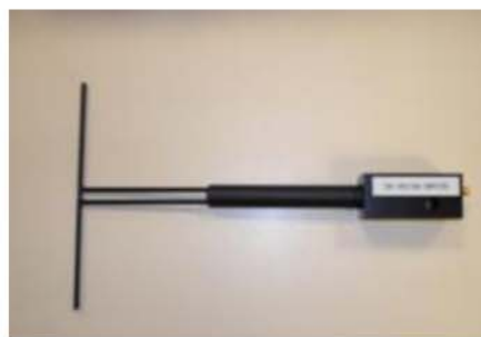
Figure 1 – Satimo COMOSAR Validation Dipole
