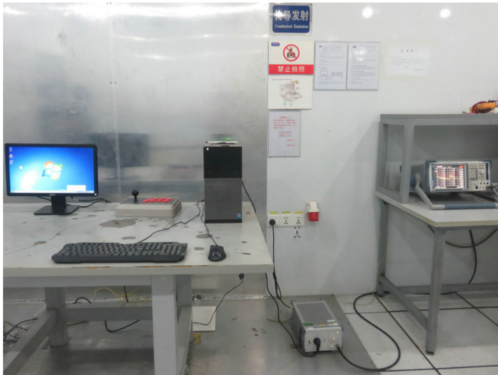
Photo of Conducted Emission Measurement
