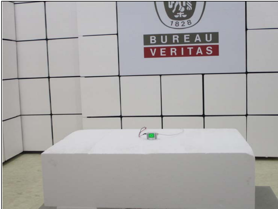
Radiated Emission below 1GHz Test
