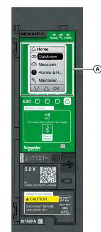
A NFC wireless communication zone
