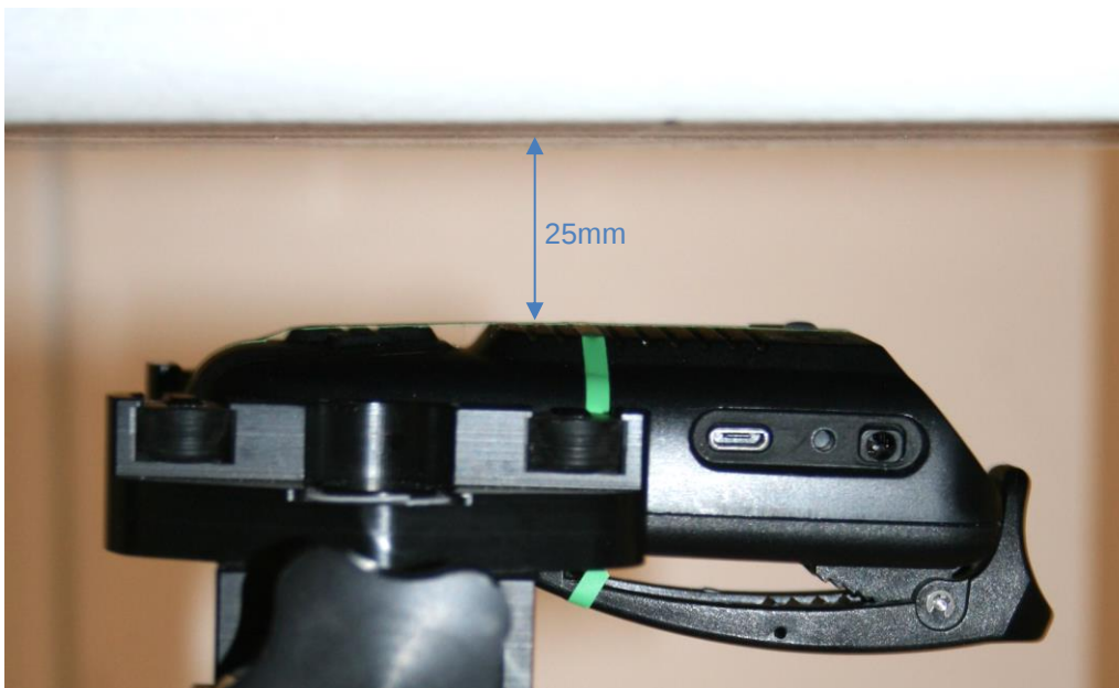
Test position "Front". DUT with front side towards the phantom with 25mm separation
