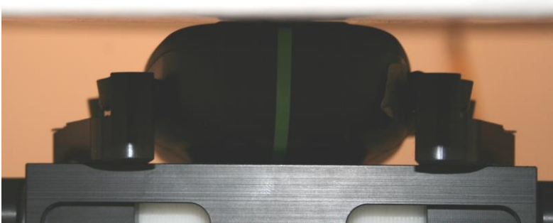
Test position "Back".DUT with back side towards the phantom with 0mm separation
