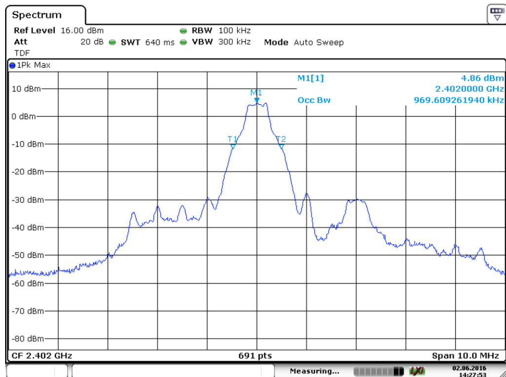
Figure 84. Low channel 99% Occupied Power Bandwidth (1 Mbps).
