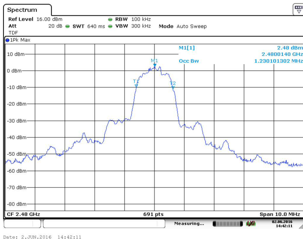
Figure 92. High channel 99% Occupied Power Bandwidth (3 Mbps).
