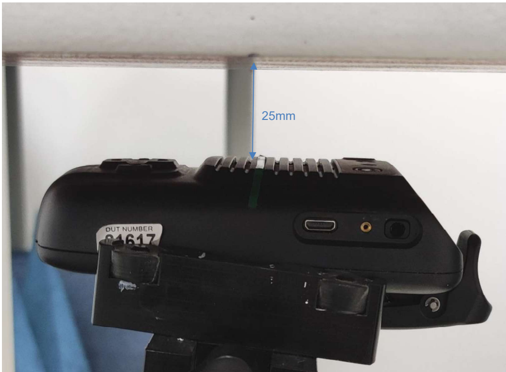
Front side of the device against the phantom, 25mm separation distance
