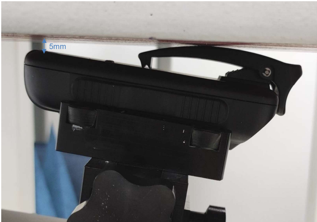
Back side of the device against the phantom, 5mm separation distance
