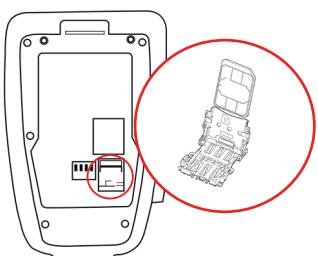
Slide the SIM card holder downward, lift the holder into an upright position and slide the SIM card into the holder. Make sure the SIM card's gold contacts face into the device and the angled corner of the card is positioned correctly (as shown in the picture on the left). Set back down the SIM card holder and slide it upwards to secure it (the SIM card should be lying flat on the device).
