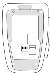
Make sure the inside of the device is clear of any dust and dirt, specially the grey area shown, to ensure the water-tightness of the device.
