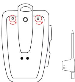
Turn off the device. Open the battery cover with the provided screwdriver and remove the device's battery.
