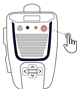
Turn on by pressing the Power button until the green LED turns off. Turn off by first pressing the Power button until "Shutdown?" appears on the screen, and then press the right arrow button to confirm the shutdown process. You can also shutdown the device through the main menu.
