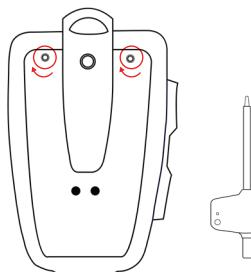
Insert the battery back into the device so that the battery contacts align and the battery label faces into the device. Then slide the battery cover back into place and screw it shut. Do not over tighten.
