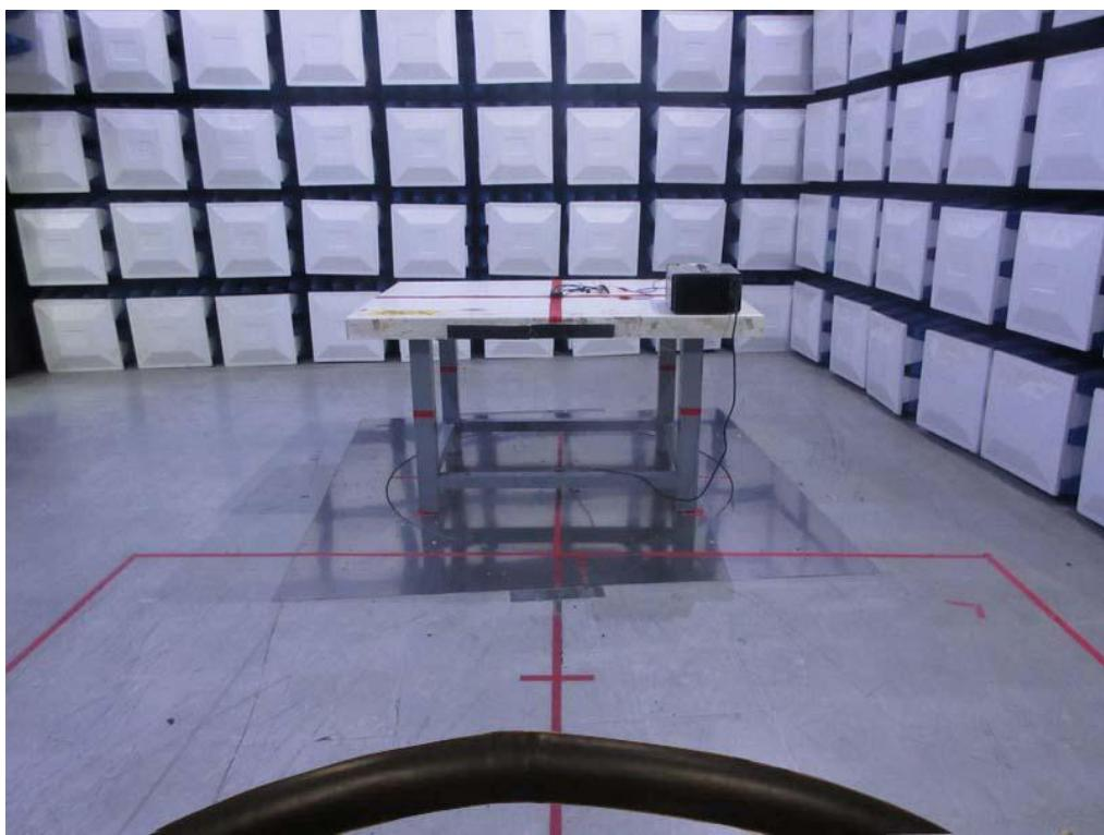
**Radiated Emissions Test Photos****30 MHz to 1000 MHz**
