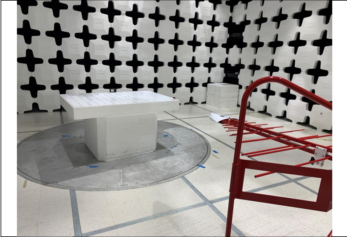
Radiated Emissions Below 1GHz setup – Front
