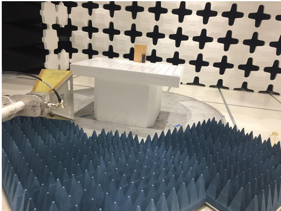
Radiated Emissions Above 1GHz setup for unintentional radiator – Front
