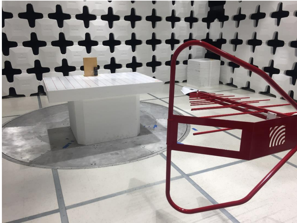
Radiated Emissions Below 1GHz setup – Front
