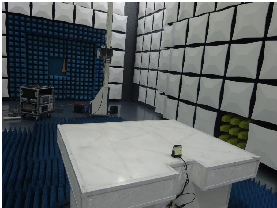
SET UP FOR RADIATED EMISSION TEST (above 1GHz)
