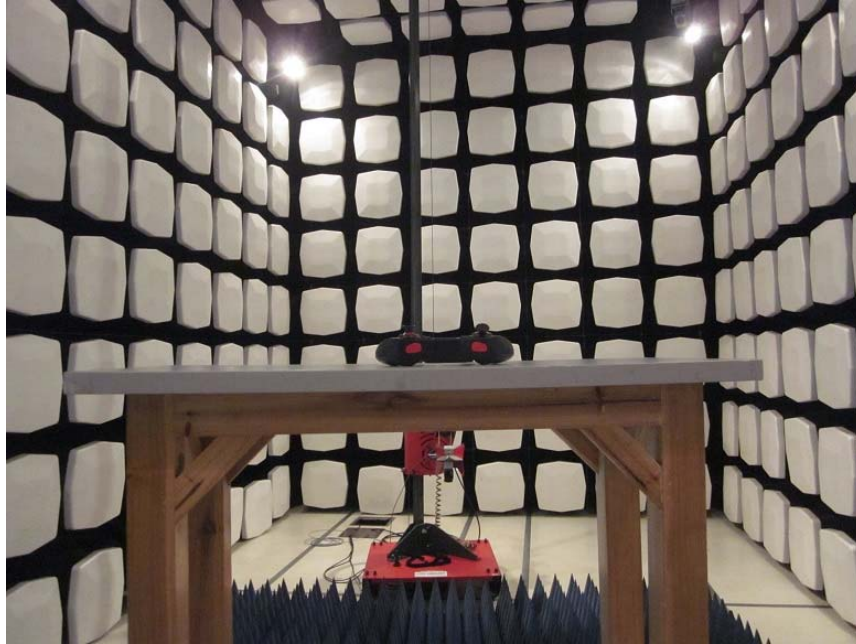
Measurement of Radiated Emission Test Set Up
