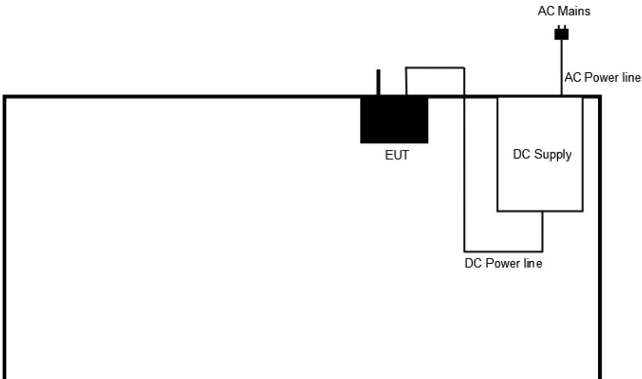
**Test Setup Diagram - Radiated Emission Test**
