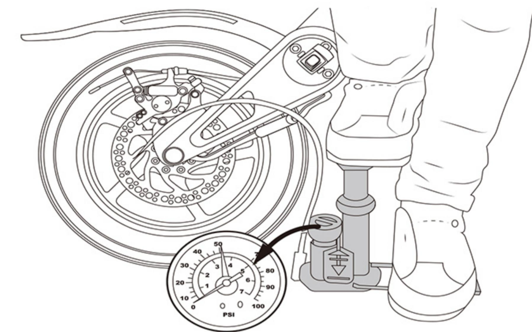
1. Using a bicycle-style tire pump equipped for a Schrader-type valve, inflate the front tire to the correct PSI indicated on the sidewall of the tire. Suggested pressure is **3.5psi to 3.8psi**.
