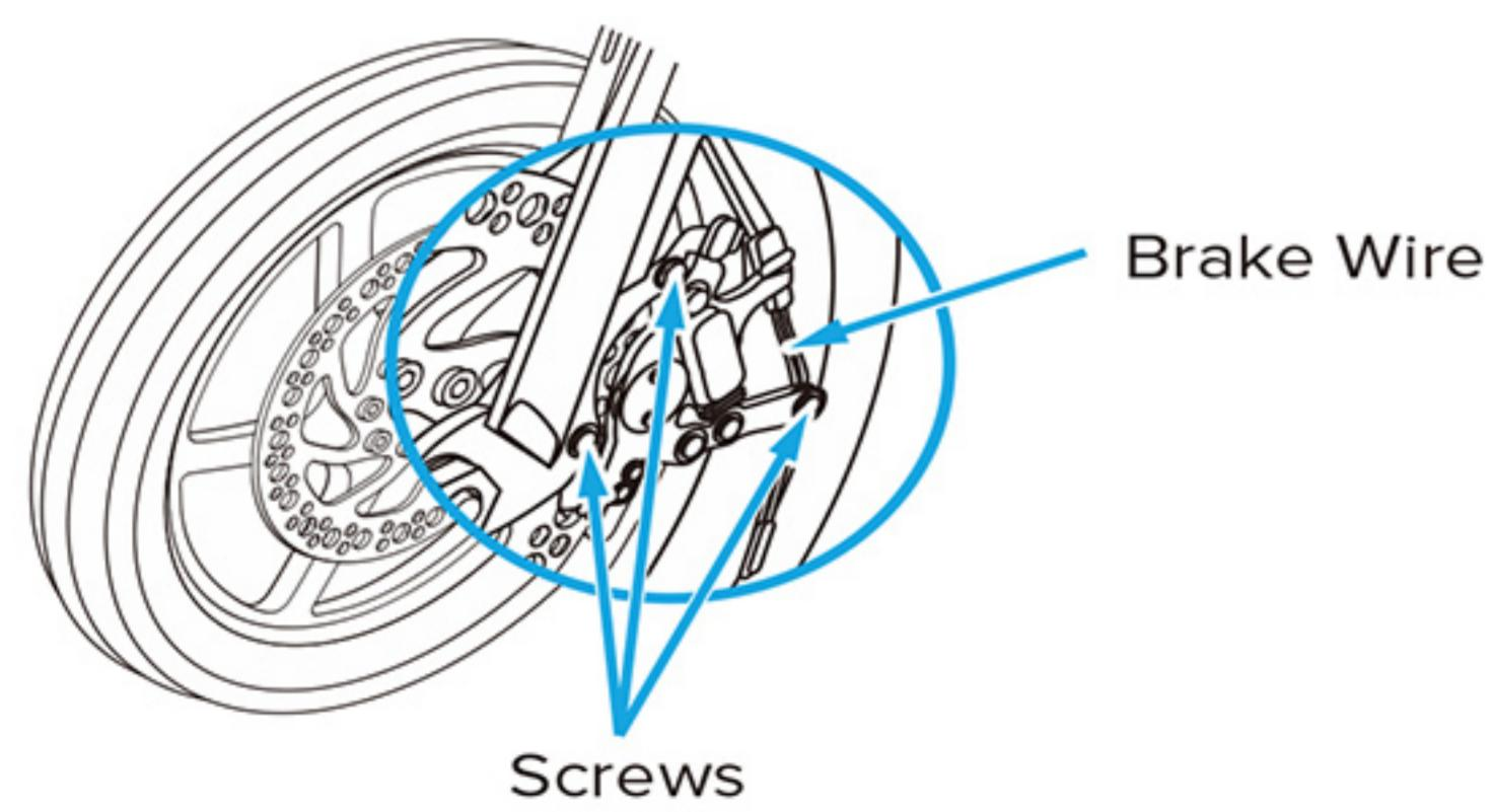
1. Loosen screws, pull out brake line and remove the braker.
