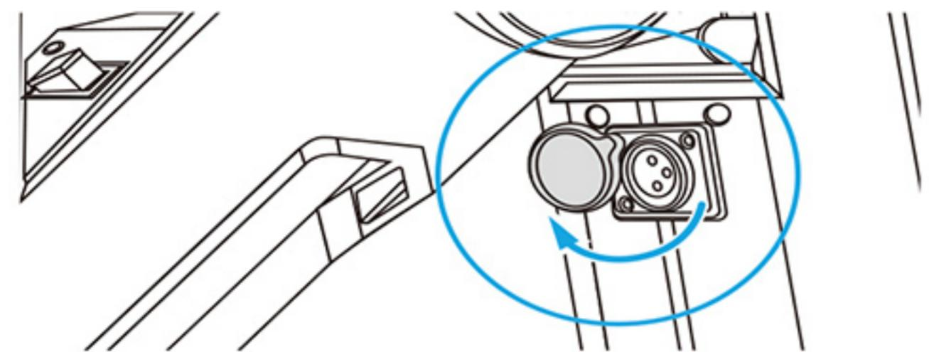
Turn the battery dustproof cover by 90 degree clockwise and you will see the charge interface
