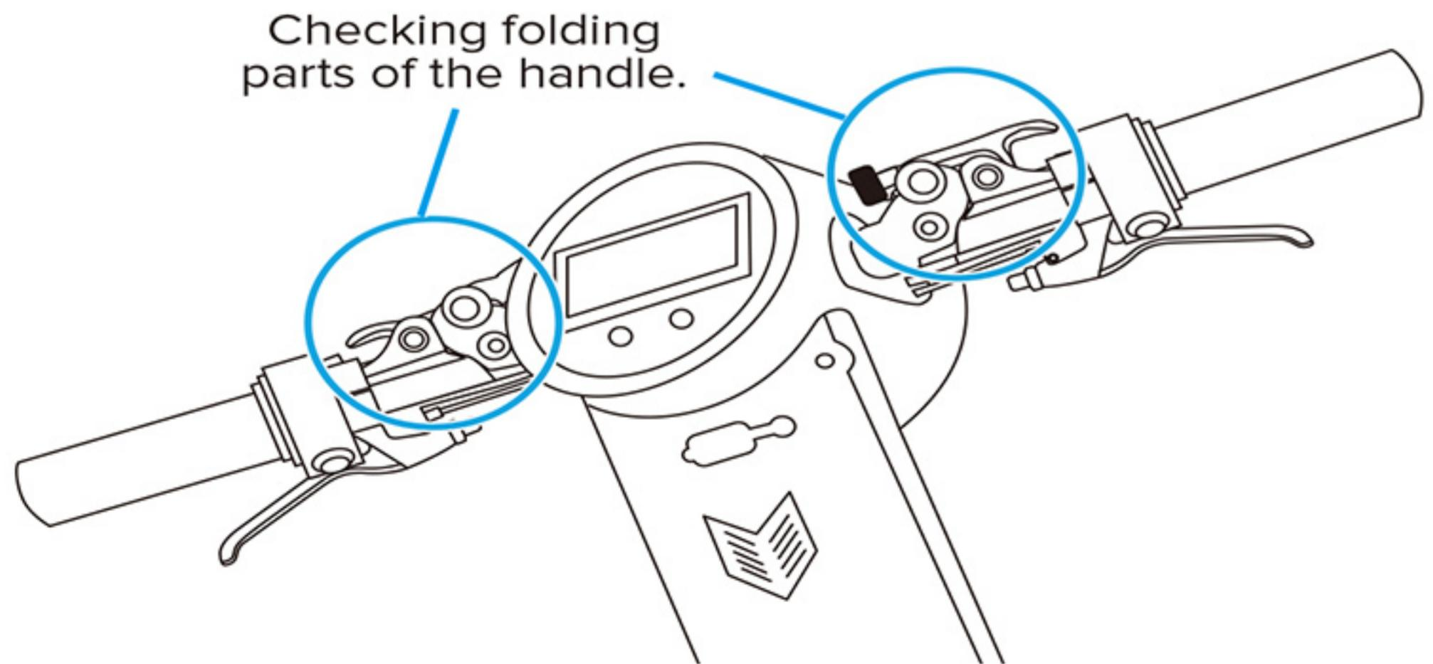
2. Checking folding frame of the bike.
