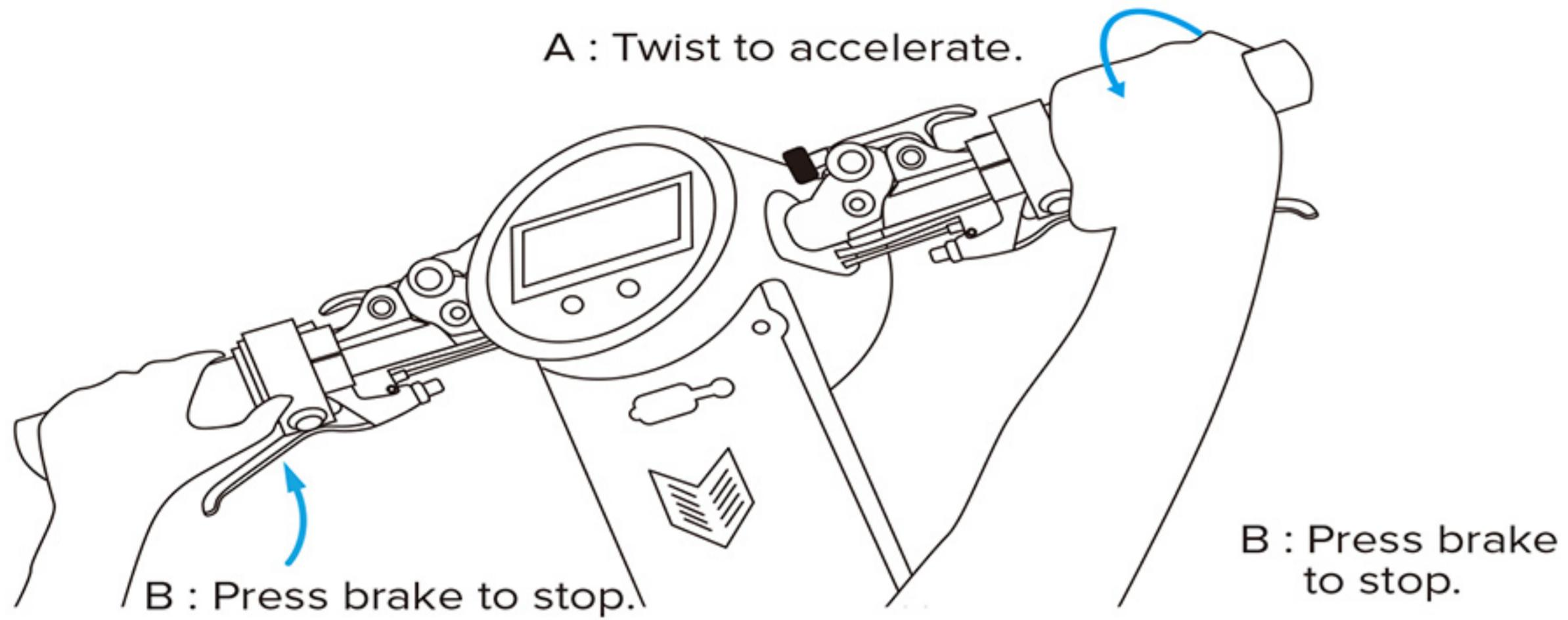
**Twist accelerator bar to drive.**
