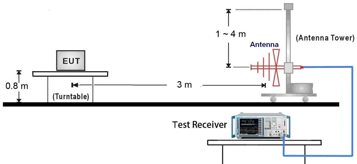
1GHz ~ 18GHz Test Setup:
