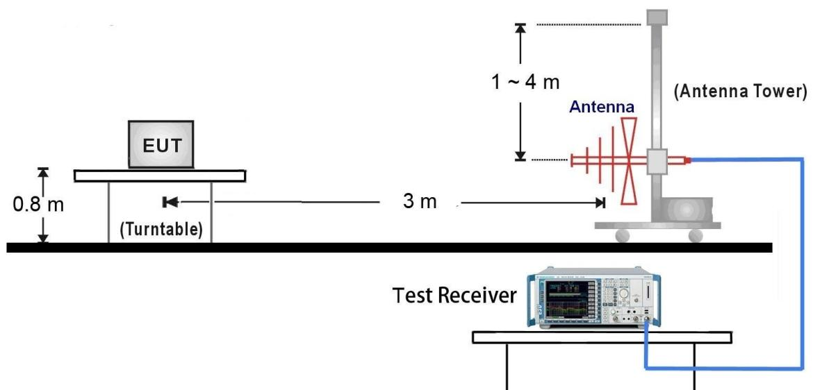
1GHz ~ 18GHz Test Setup:
