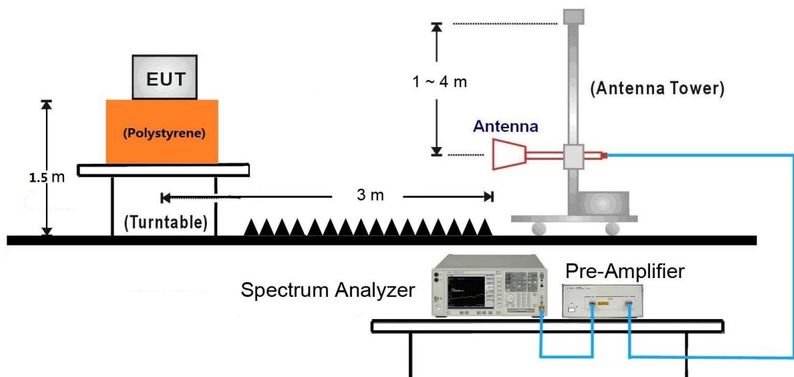
18GHz ~25GHz Test Setup:
