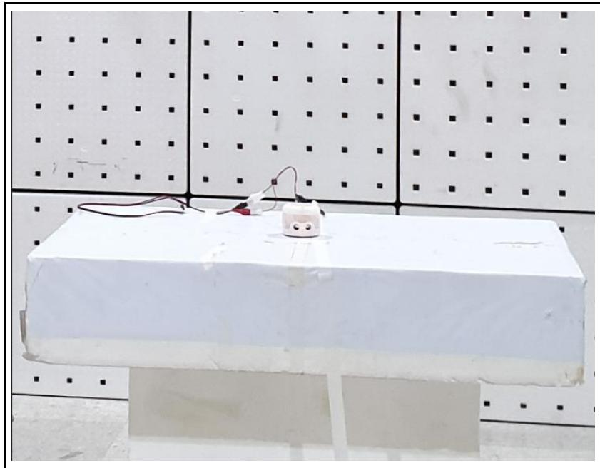
**2. Photo of Radiated Spurious Emission Test (Below 1 GHz)**
