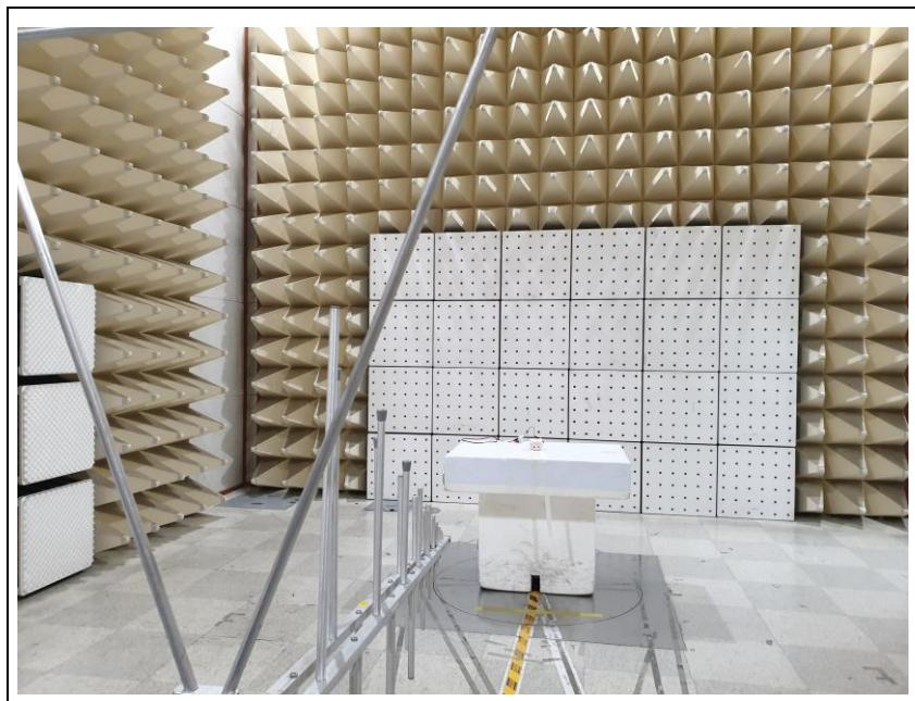
**3. Photo of Radiated Spurious Emission Test (Above 1 GHz)**
