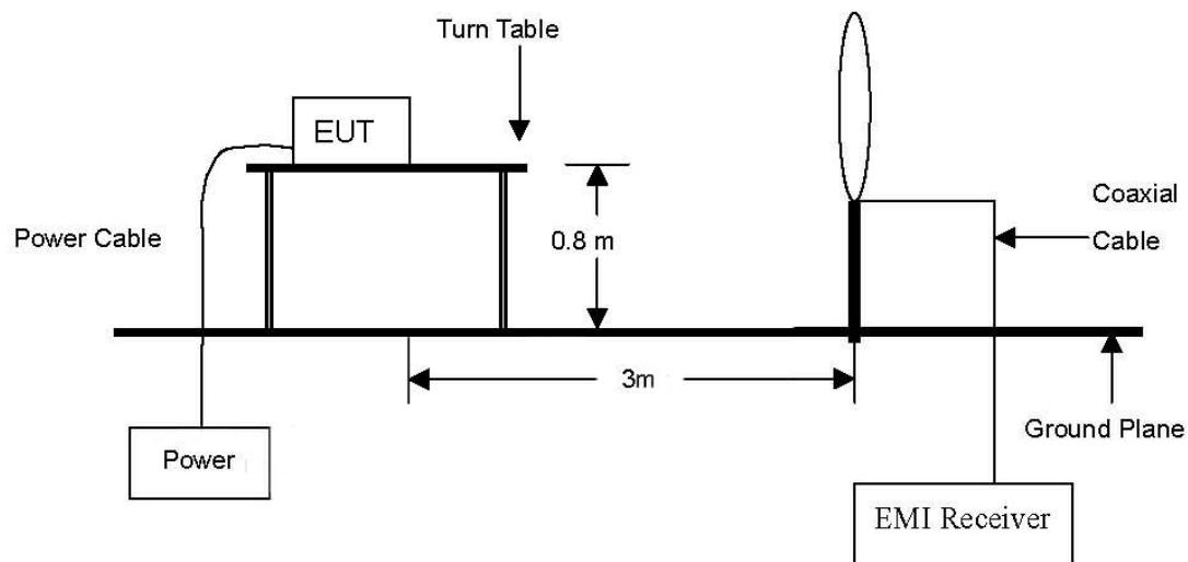
The diagram below shows the test setup that is utilized to make the measurements for emission from 30 MHz to 1 GHz.
