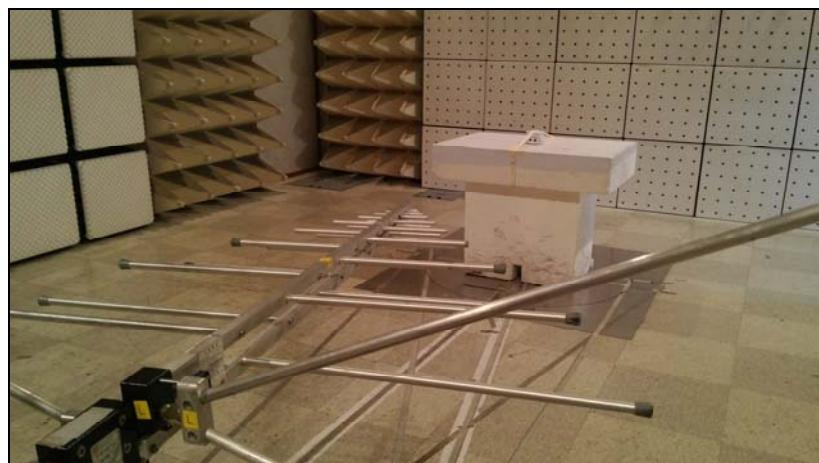
**B. Photo of Radiated Spurious Emission Test (Above 1 GHz)**
