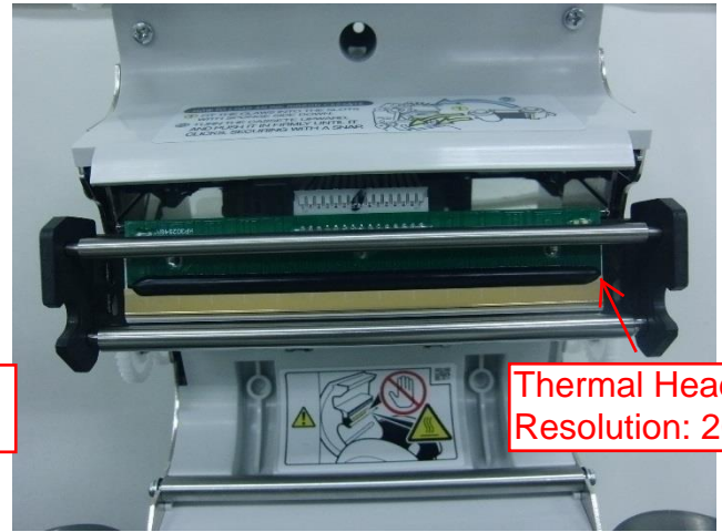
Fig.8. CPM-100G5U Thermal head focus
