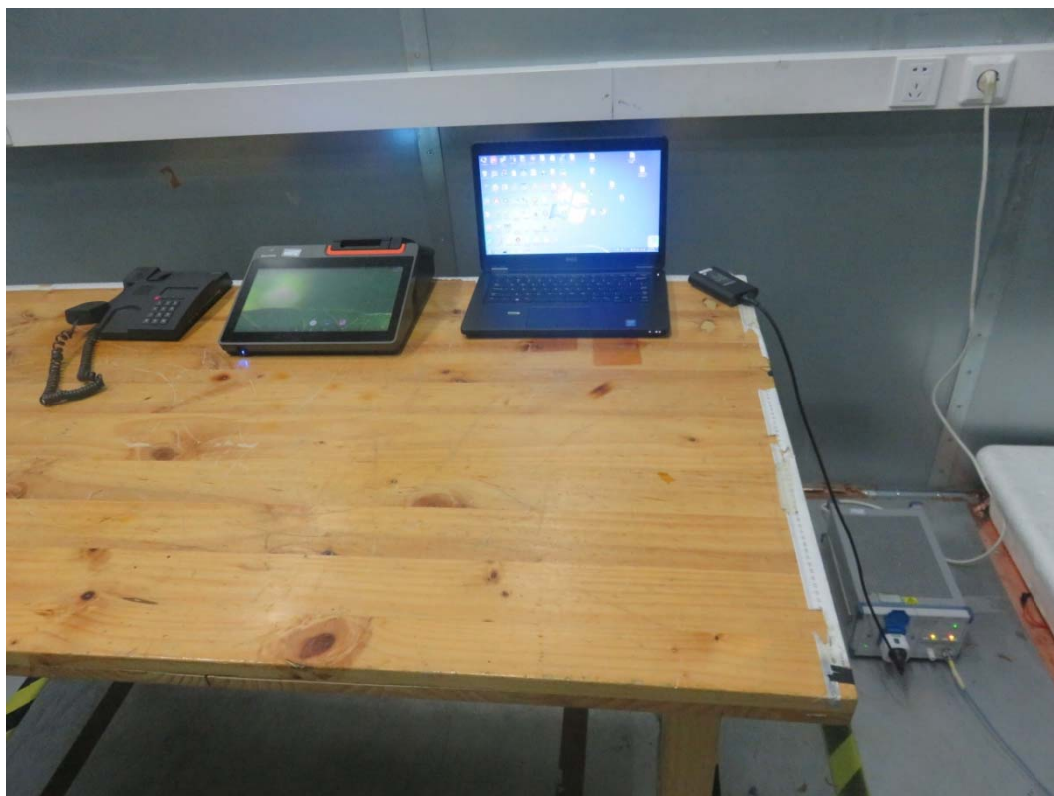
Picture 3 Conducted Emission Test Setup
