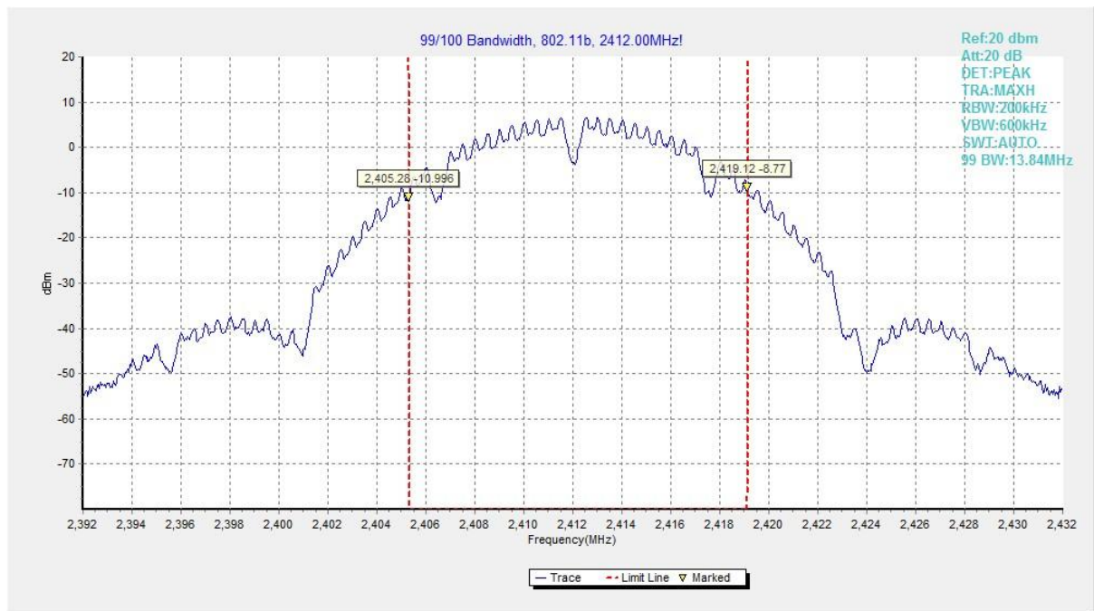
Fig.70 99% Occupied Bandwidth (802.11b, CH 1)
