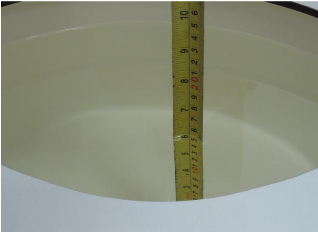
Picture C.4: Liquid depth in the flat Phantom (2450 MHz) (15.2cm deep)
