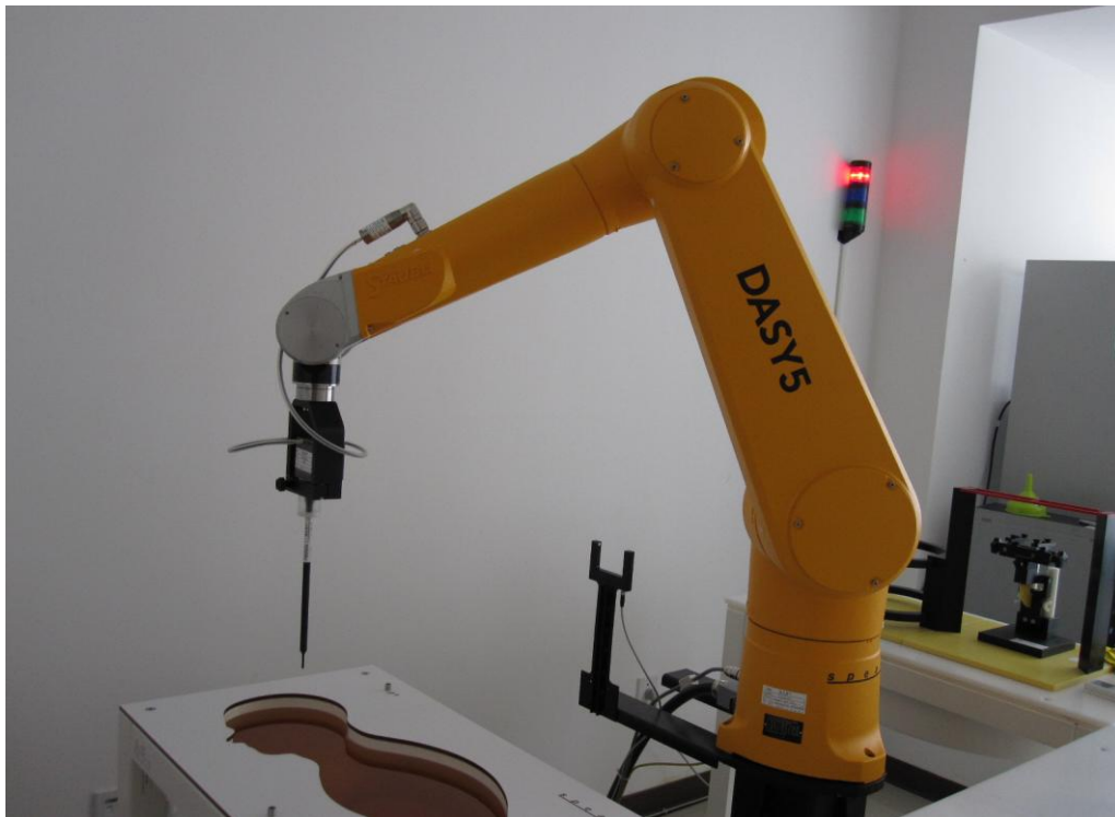
Picture C.1: Specific Absorption Rate Test Layout
