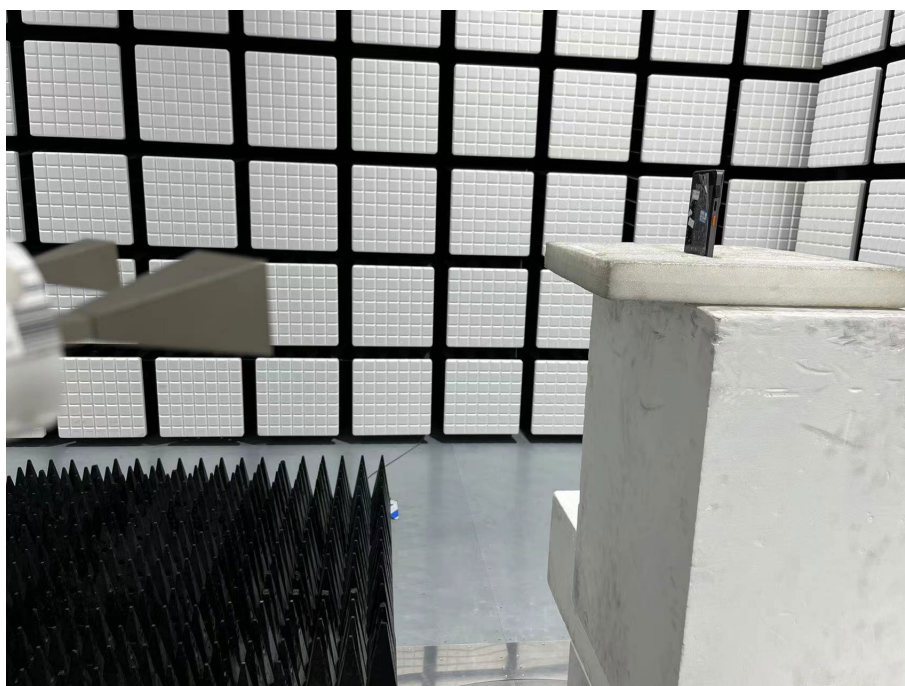
Description: Radiated Emission Test Setup (Above 18GHz)
