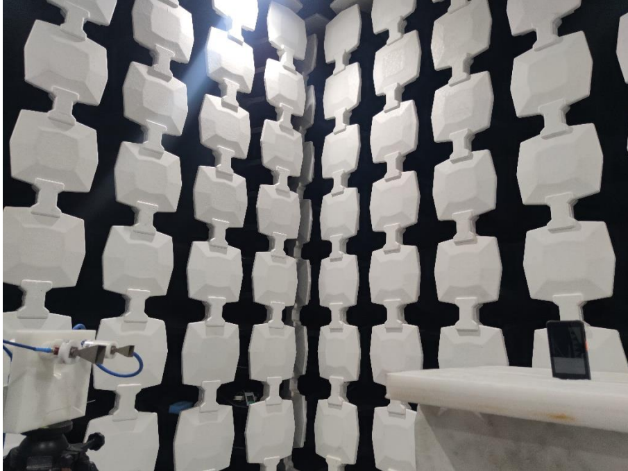
Description: Radiated Emission Test Setup (Above 18GHz)
