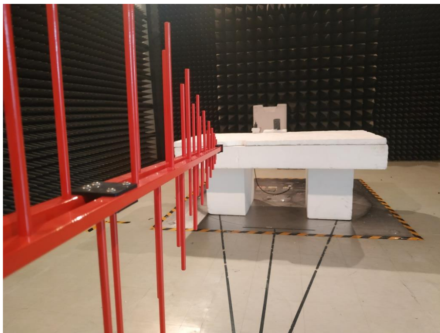
Radiated Emissions View (1GHz-18GHz)
