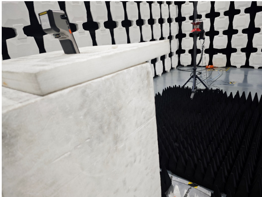
Description: Radiated Emission Test Setup (Above 18GHz)
