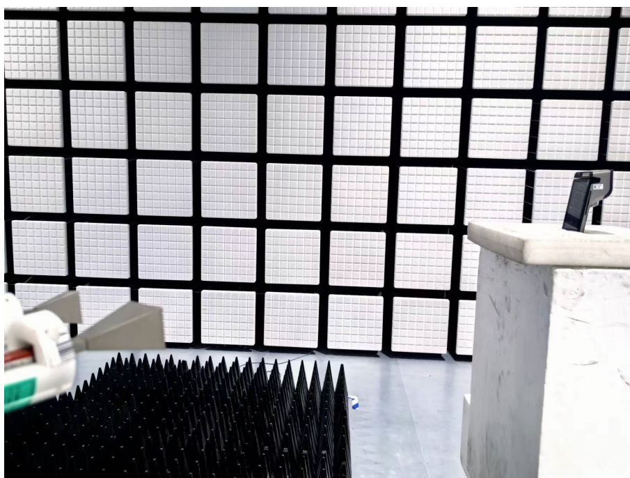
Description: Radiated Emission Test Setup (Above 18GHz)
