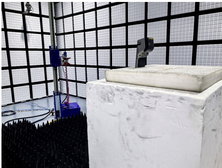
Description: Radiated Emission Test Setup (Above 18GHz)
