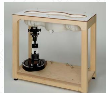
Figure 7.4.5-1: SAM Twin Phantom
