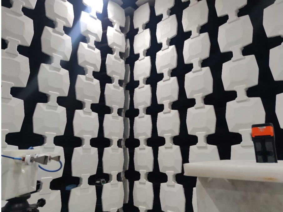
Description: Radiated Emission Test Setup (Above 18GHz)
