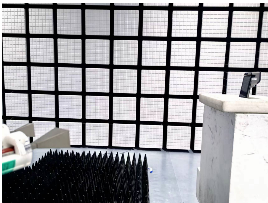
Description: Radiated Emission Test Setup (Above 18GHz)
