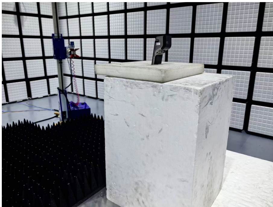
Description: Radiated Emission Test Setup (Above 18GHz)
