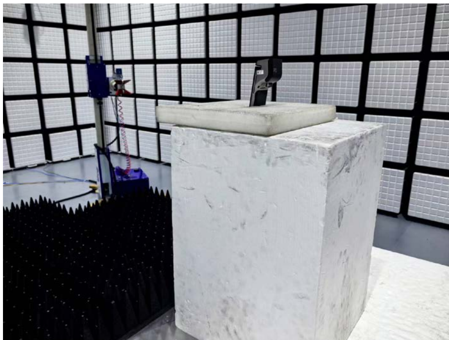
Description: Radiated Emission Test Setup (Above 18GHz)
