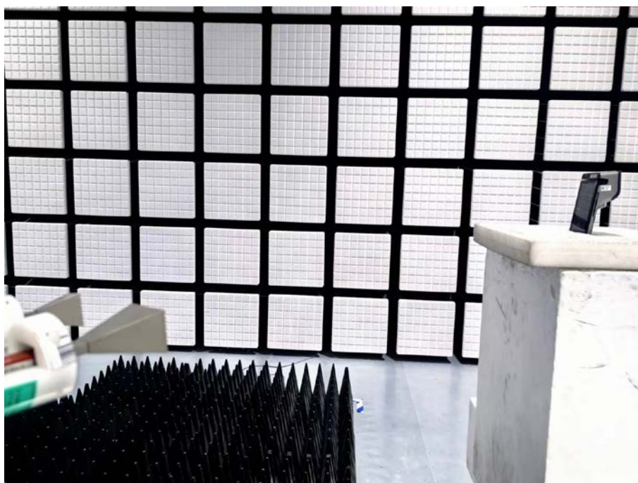
Description: Radiated Emission Test Setup (Above 18GHz)
