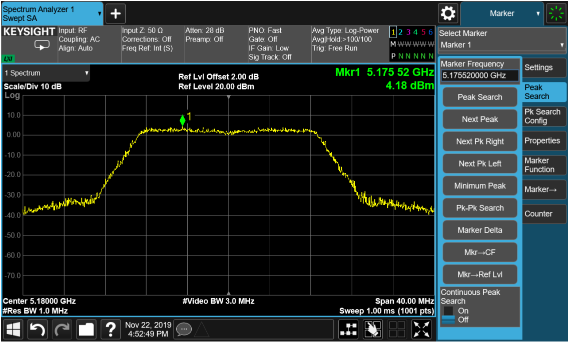
Figure 22: Power Spectral Density, 802.11n(HT20), 5180MHz
