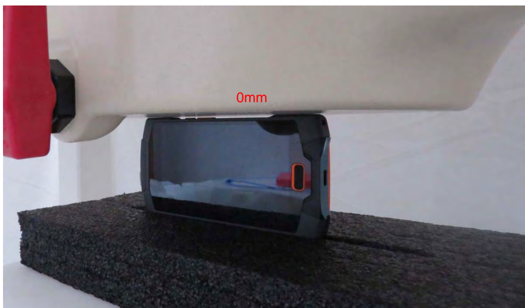
Picture 8: Right Side, the distance from handset to the bottom of the Phantom is 0mm
