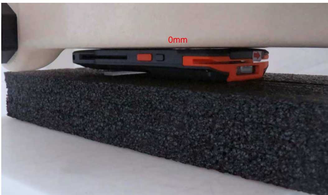
Picture 6: Front Side, the distance from handset to the bottom of the Phantom is 0mm
