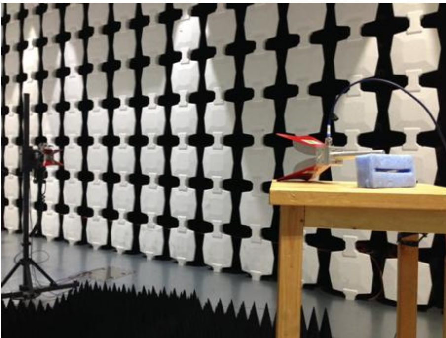
Description: Substitution Antenna for EIRP Test
